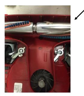
The pictures below show the beater bar correctly aligned so the belt goes over the belt guide
