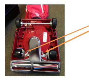
There are 2 latches on the bottom that hold the silver/metal plate in place.
