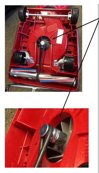
The first area that will cause a problem is the motor peg that the belt attaches.
