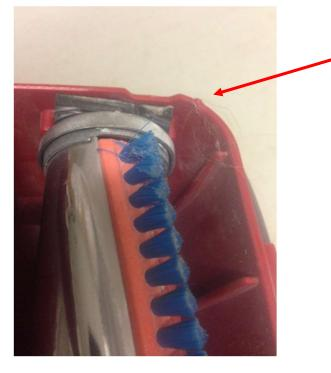
If the beater bar is installed correctly the flat part will be on top
